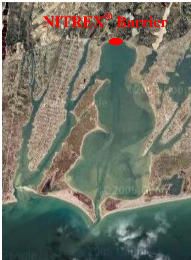
Figure 1. The Nitrex Permeable Reactive Barrier is located at the head of Waquoit Bay in Falmouth, MA. The Barrier begins 0.5 meters below the surface and continues for 2 meters. The barrier is 3.5 meters wide and stretches along the beach for 16.5 meters. The photograph here was taken from googlemaps.com, October, 2005.
