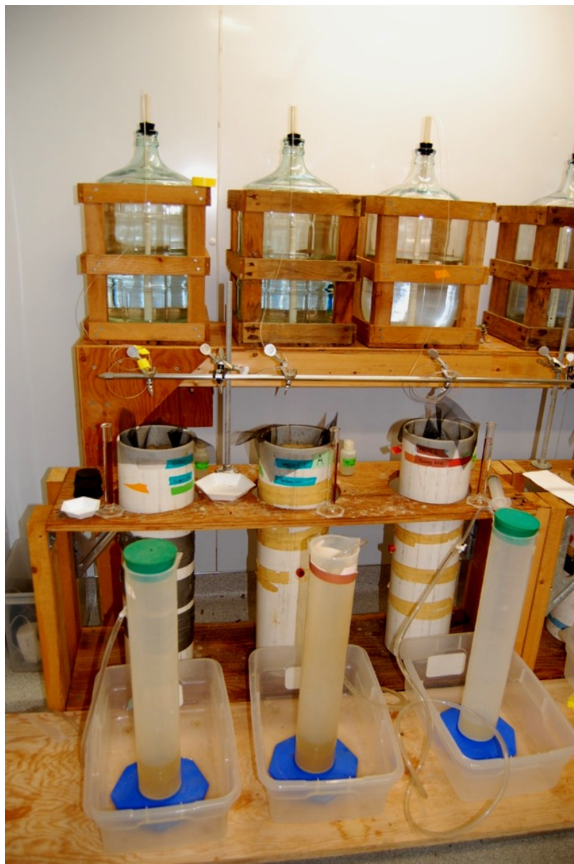
Fig. 5. Microcosm setup including the Mariotte bottle (carboy), tubing into the PVC pipe, the pipe containing wood chips and sand, and tubing from the pipe into a graduated cylinder.
